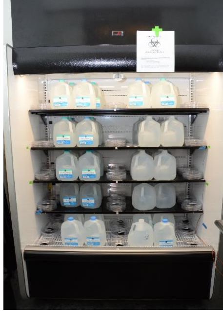
Figure 4. Commercial refrigeration unit loaded as per manufacturer’s instruction and stocked with inoculated powder-coated coupons
